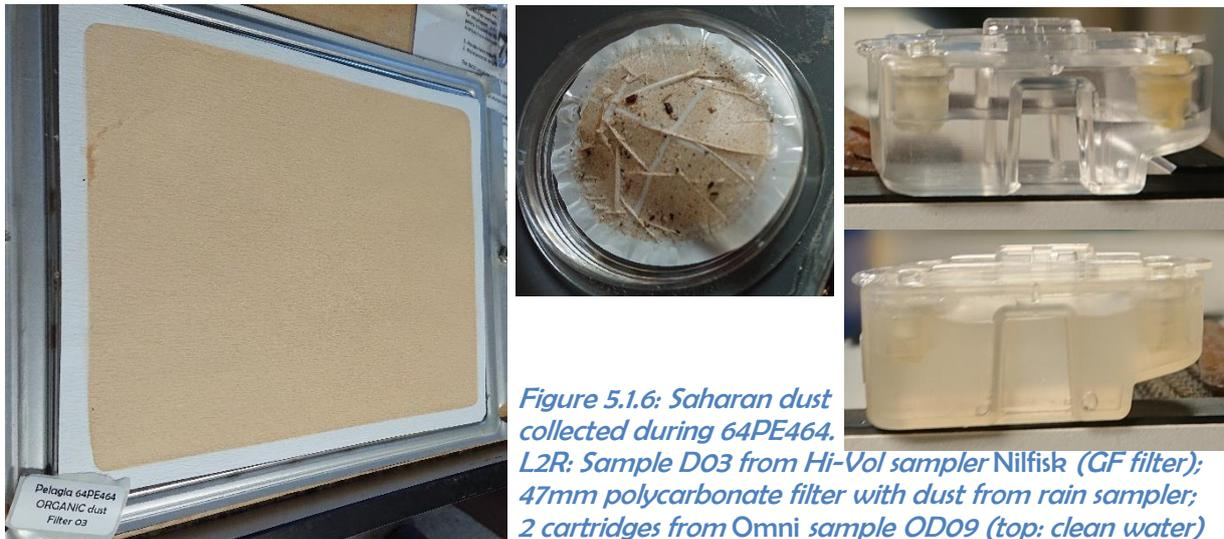
Figure 5.1.6: Saharan dust collected during 64PE464. L2R: Sample D03 from Hi-Vol sampler Nilfisk (GF filter); 47mm polycarbonate filter with dust from rain sampler; 2 cartridges from Omni sample OD09 (top: clean water)
