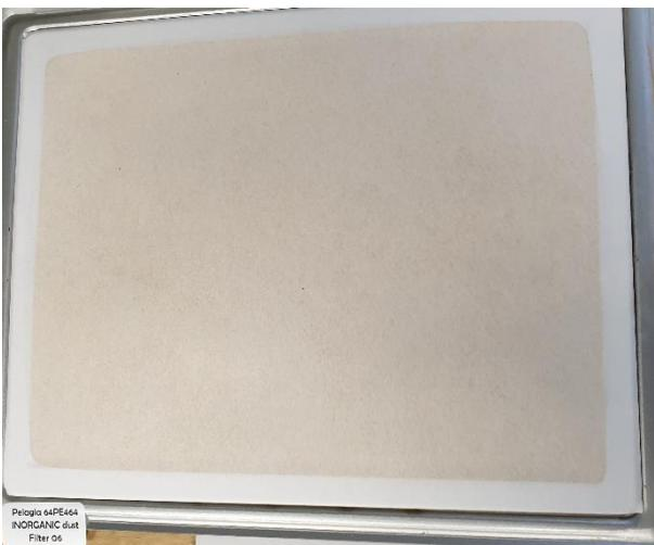
Figure 4.5: Saharan dust collected on a glass-fibre filter and showing the characteristic orange colour.
