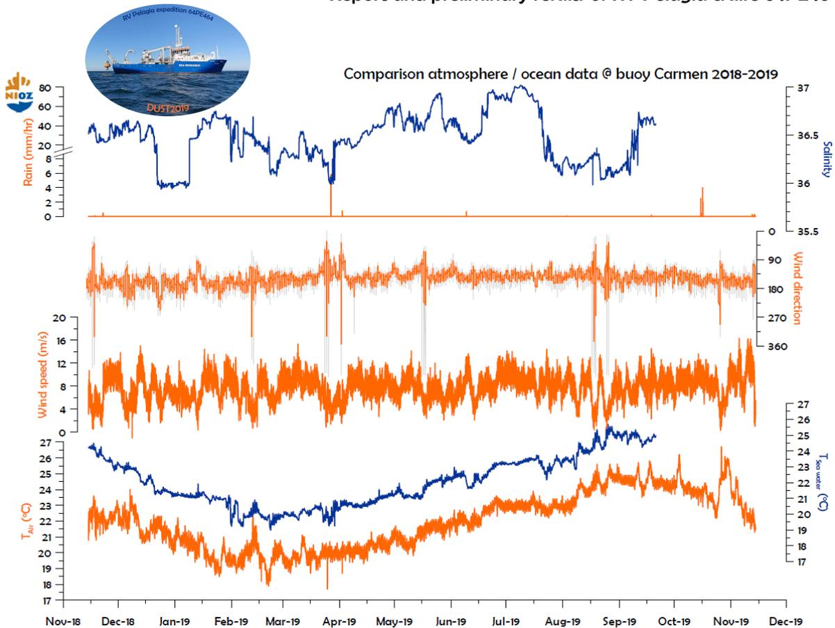
Figure 5.2.1: timeseries of buoy Carmen from November 2018 – November 2019. Blue graphs [salinity and water temperature] from sea-surface CTD, orange graphs [rain, wind direction, wind speed and air temperature] from VAISALA® meteorological sensor.
