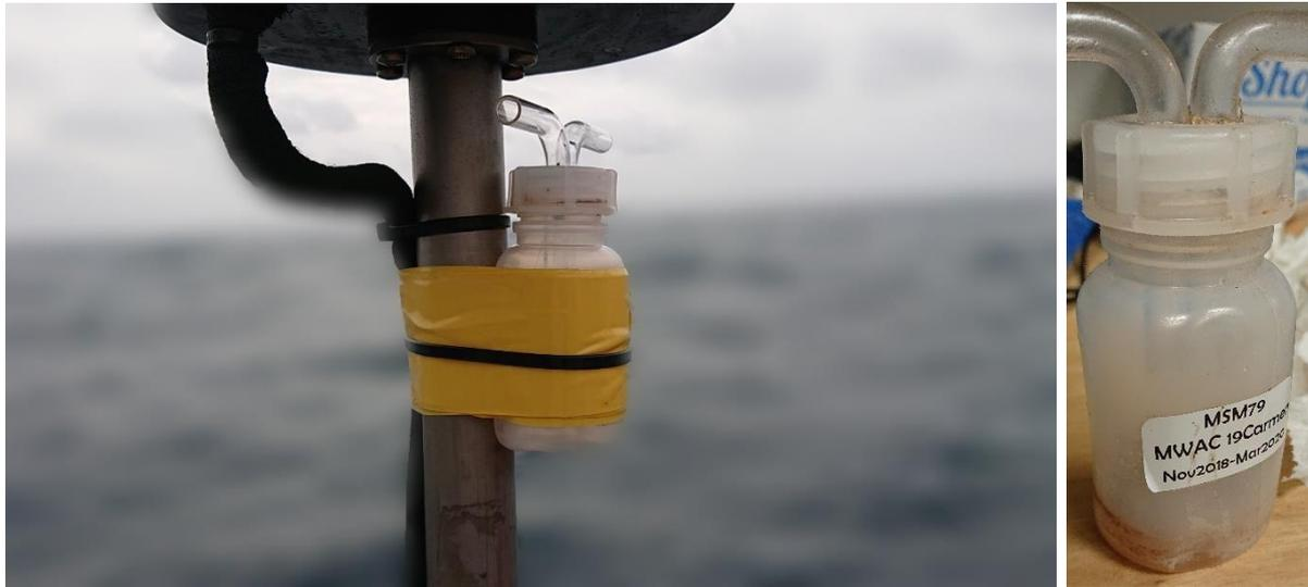
*Figure 5.2.3: MWAC sampler on buoy Carmen, positioned directly underneath the inlet through which air is being pumped into chimney, which is connected to the filter cups. The air vane on the buoy guarantees that the MWAC's opening is directed into the wind.*
