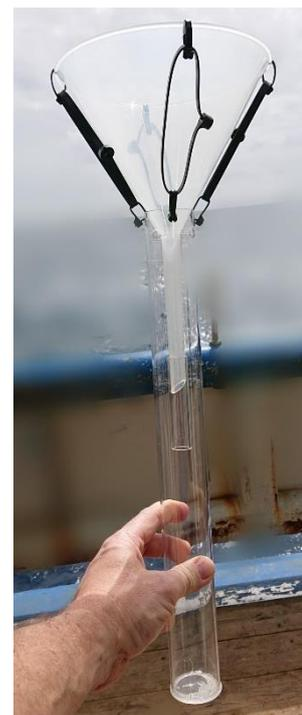
Figure 4.7: Prototype wet-dust collector, to be assembled on buoy *Laura*.
