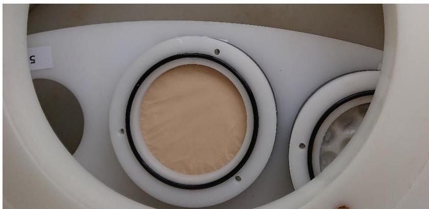
Figure 5.2.2: filter nr 4 of time series 19Carmen, on the carousel inside the buoy, showing the typical orange colouration caused by Saharan dust.
