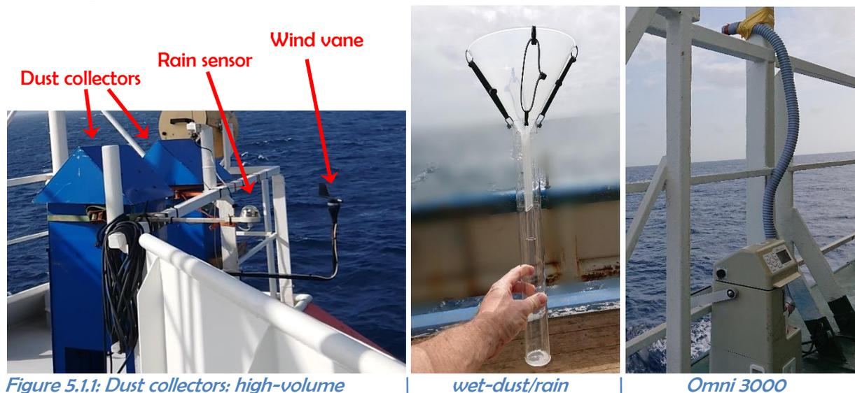
Figure 5.1.1: Dust collectors: high-volume
